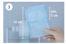
All test strips must have two seal seams separated by a gap of at least 5 cm.
