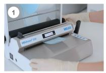
Cut three 10 cm test strips from the smallest packaging format used in the practice.
